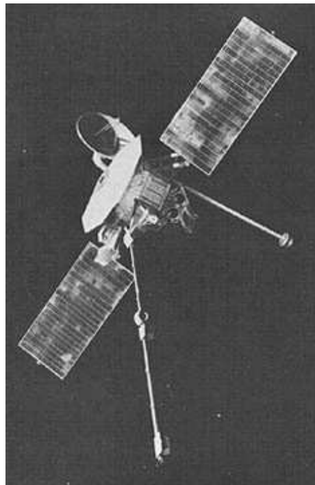
Fig. 4-2. Alternatively, they could be rotated away from the Sun along the long axis. This was the method chosen because it allowed nitrogen gas thrusters to be mounted at the tips of the panels, thus attaining more efficiency in orienting the spacecraft.
