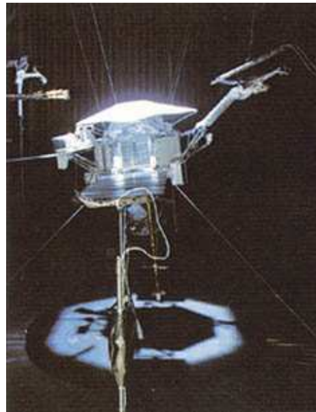
Fig. 4-3. The flight sunshade proved effective in protecting the spacecraft from solar heating generally.
