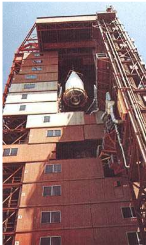
Fig. 4-13. At last Mariner Venus/Mercury, within its protective shroud, is hoisted up the gantry for mating with the Atlas/ Centaur launch vehicle.
