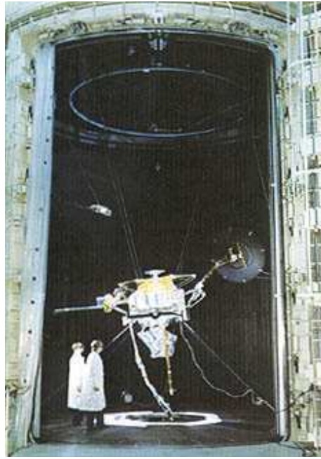
Fig. 4-9. Final space simulation tests took place at JPL, where the spacecraft went through a series of exercises under conditions of vacuum and solar radiation it was expected to experience in Mercury orbit.
